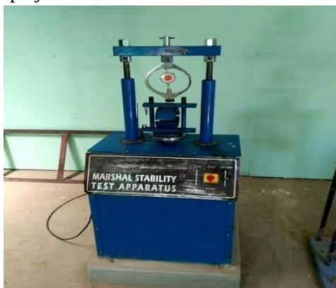
Fig. 4 Marshall Stability Test Apparatus
