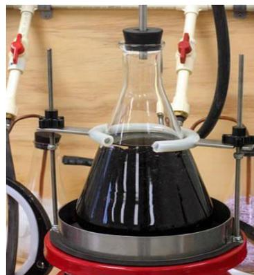
Fig. 2 Specific Gravity Apparatus
