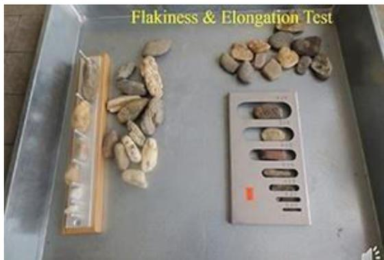
Fig. 3 Flakiness and Elongation Test Apparatus
