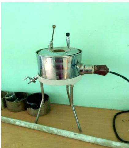
Fig. 1 Standard Viscometer
